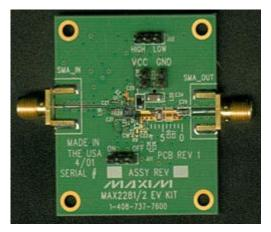
The MAX2282 is a single-supply, low-voltage linear power amplifier designed for cellular band handsets. The MAX2282 is specifically designed for use in the Japanese cellular band and offers excellent performance when tuned for CDMA. The device features a low-power mode, which provides up to +18dBm output power with higher efficiency than competitive PA's, significantly extending average talk time. MAX2282 is available in a unique tiny UCSP package, just 2.5mm x 2.5mm.
